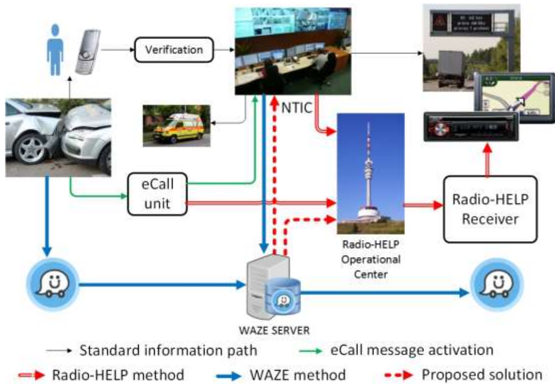
Figure 1 - Transmission and acquisition of information in the event of an accident with the use of eCall, Radio Help and WAZE (Author)
